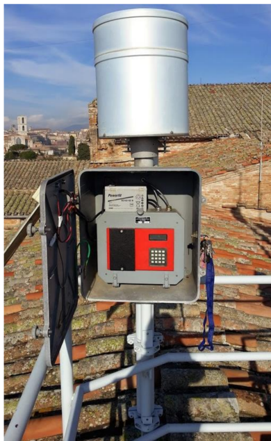
Figure 1. Rain gauge with digital data logger correctly working at Perugia (central Italy).
