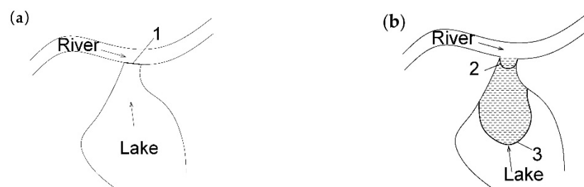
Figure 3. Schematic processing of backflow from river to lake (BRL). (a) the beginning of the BRL; (b) the processing and the influence scope of the BRL.
