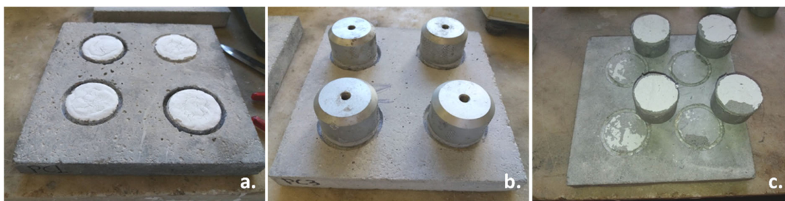
Figure S2. Steps of pull-off measurements; (a) coating applied onto the cyclical concrete surface, (b) dollies stuck onto the coating surface, and (c) dollies with coating and adhesive after the pull-off measurement.
