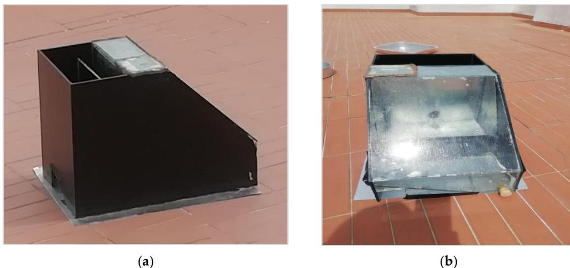
**Figure 2.** Solar still used in the field trials: (a) side view and (b) front view. The solar still is 0.50 m long and 0.30 m high and wide, respectively. The walls of the solar still were built in glass with a thickness of 5 mm and the water basin was in metal (area = 0.054 m<sup>2</sup>). It was covered with black adhesive paper to improve the absorptivity of solar radiation and increase the internal heat of the solar still.
