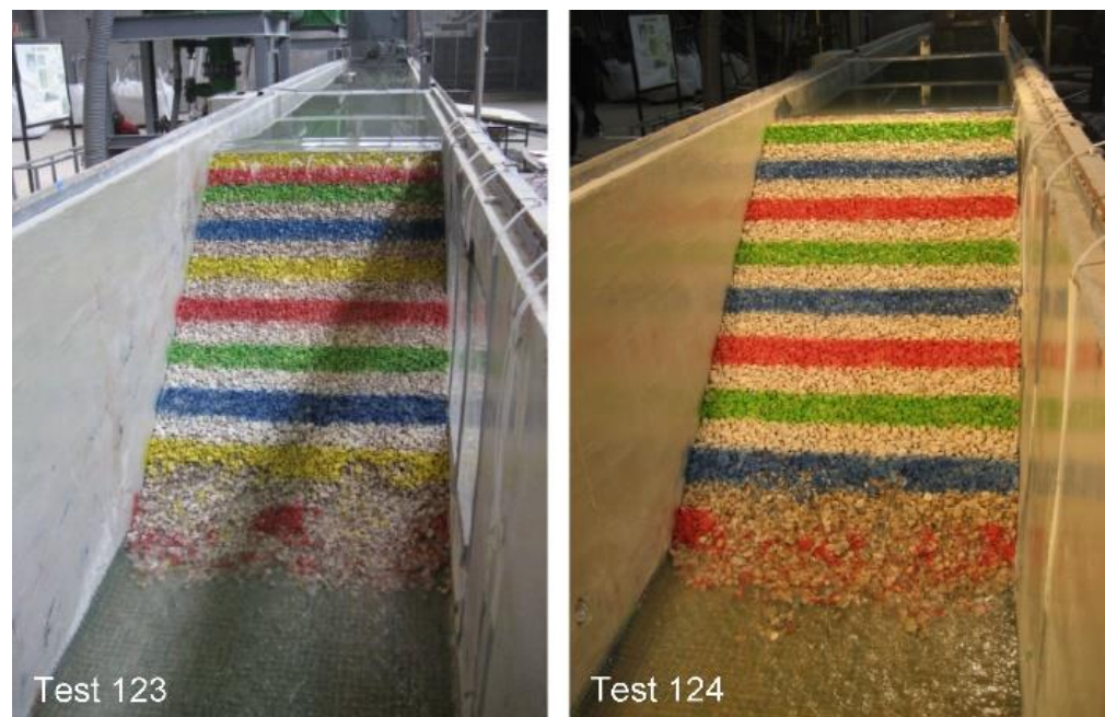
Figure 17. Failure progress in tests n° 123 and 124 for a discharge of roughly 0.0090 \text{ m}^3 \text{ s}^{-1} .
