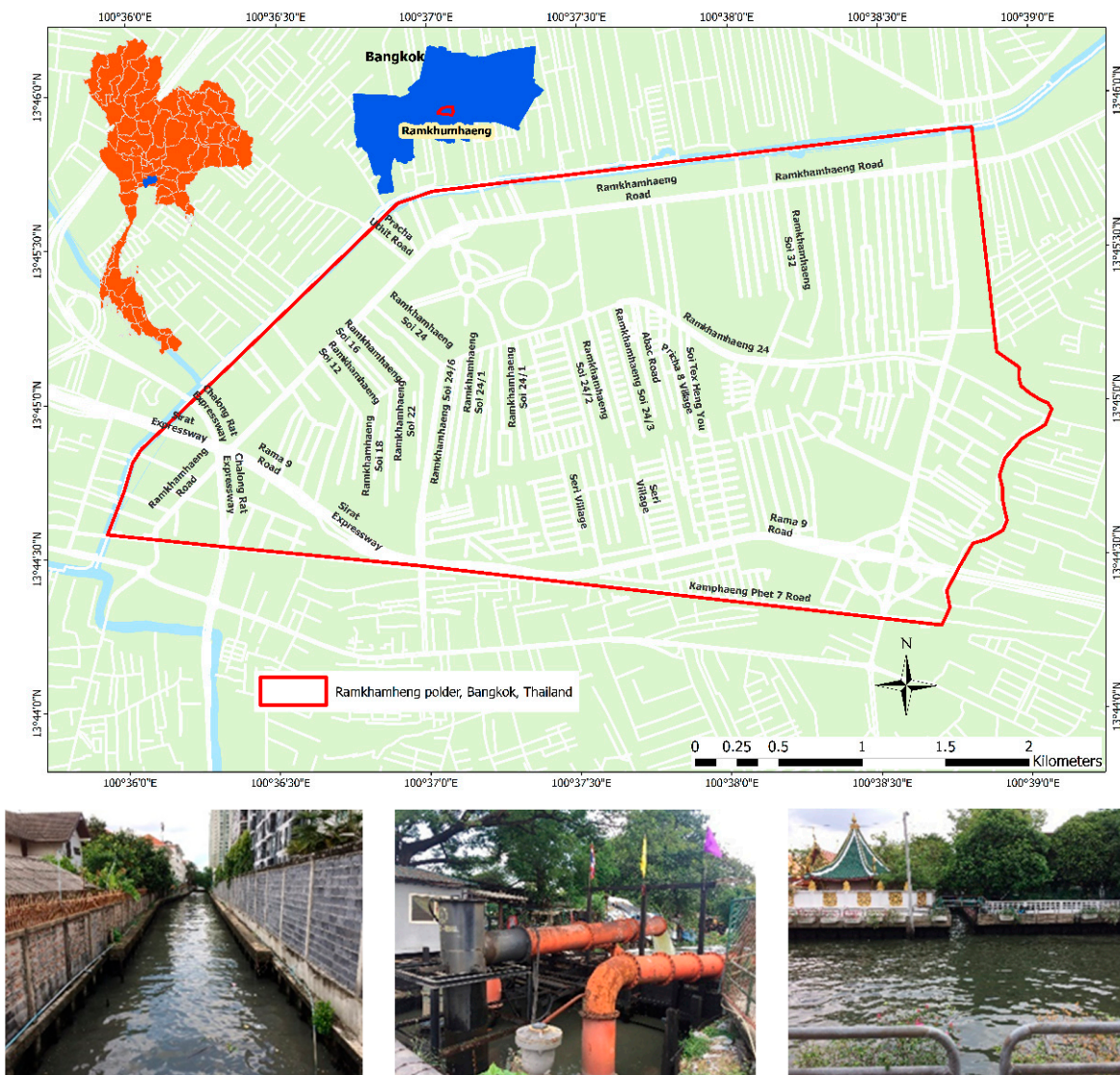
Figure 1. Top. Map of the Ramkhamhaeng polder, Bangkok, Thailand. The Ramkhamhaeng polder is one of Bangkok’s water management polder systems [51]. Additionally, shown (bottom photographs) are the typologies of the drainage system illustrating its distinct characteristics from those of the Global North. Bottom left: A secondary canal within the study area. Bottom middle: Pumping water from the central region of the study area towards the primary canal system. Bottom right: The primary canal, Saen Seab, is in the foreground, with the mouth of a secondary canal visible to the right of the temple area (photos by authors).
