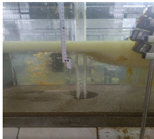
Figure 4. Local scour hole around a pier.
