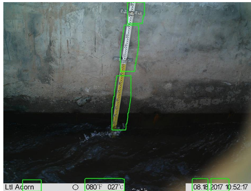
Figure 12. The effect of contour detection from the image in Figure 9b.
