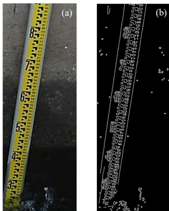
Figure 13. The effect of contour detection and edge detection. (a) is obtained from Figure 12 by the size of the area of the detected contour. (b) The effect from (a) by the edge detection of Canny operator.
