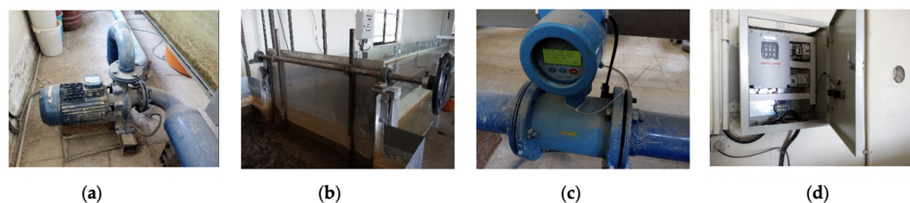
Figure 2. Some experimental equipment used for this experimental study: (a) electromotor pump; (b) slide-gate at the end of the flume; (c) variable frequency drive; (d) electromagnetic flowmeter.
