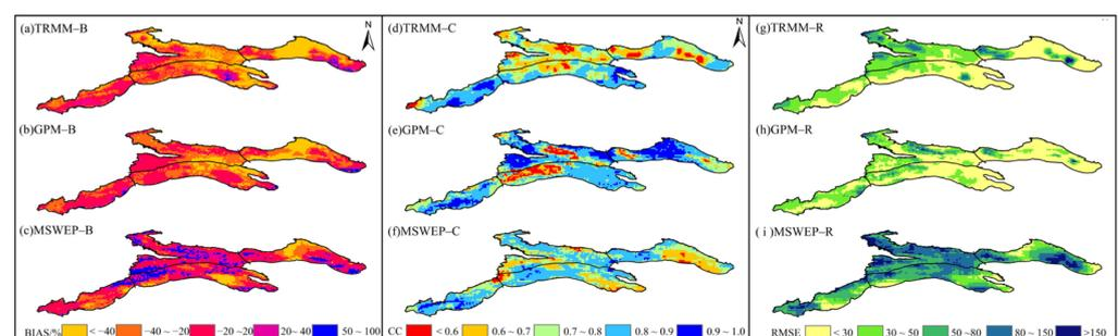
**Figure 10.** Spatial distribution of BIAS (a–c), CC (d–f) and RMSE (g–i) between precipitation products and measured precipitation interpolation results. TRMM (a,d,g); GPM (b,e,h); MSWEP (g–i).
