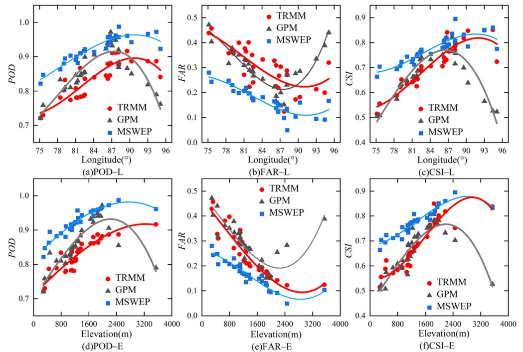
**Figure 11.** Scatter diagram and fitting lines of daily precipitation detection indicators and longitude (a–c) and elevation (d–f) of three products.
