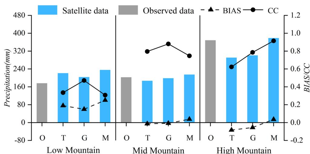
**Figure 13.** Comparison of average precipitation of three sets of satellite products in different elevation zones. Note: Measured data, TRMM, GPM and MSWEP are in turn from left to right in each elevation zone.
