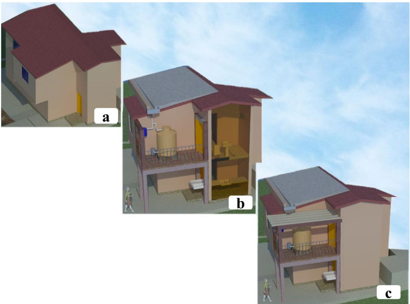
**Figure 9.** Proposed modifications to the pattern single-family household based on installing the rainwater harvesting system. (a) SFH original condition, (b) Detail of RWHS installation, (c) SFH final volumetry.
