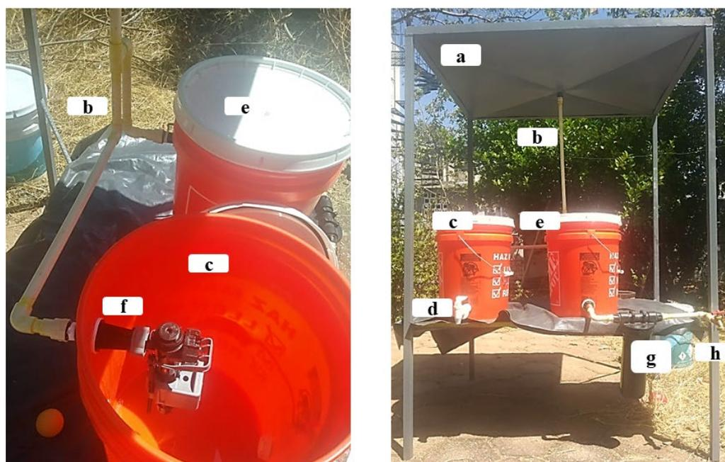
**Figure 5.** In situ rainwater harvesting sampling system. (a) Catchment surface area; (b) conveyance; (c) first-rain separator; (d) separated effluent outlet; (e) rainwater storage; (f) Kerick valve; (g) filter; (h) treated effluent outlet.
