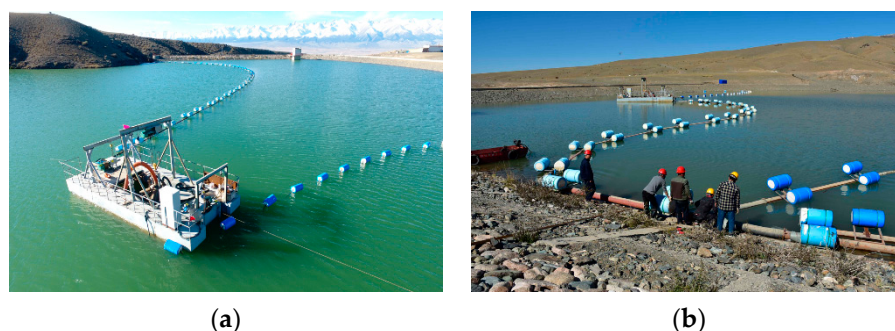
Figure 1. Field test of self-priming pipe sand removal technology. (a) Field test of reservoir desilting, (b) Desilting pipe.
