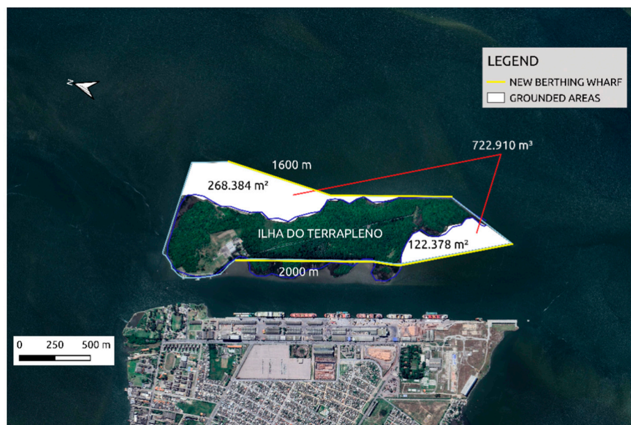
Figure 13. Ilha do Terrapleno. Dark blue (cyan) contour represents the actual (proposed) configuration for the island. White areas indicate the island expansion due to the proposed configuration. Yellow lines indicate the linearized coastline for mooring operations.
