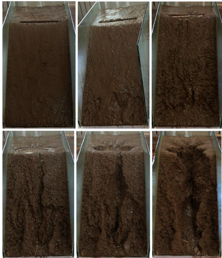
Figure 4. Process of soil erosion under rainfall.
