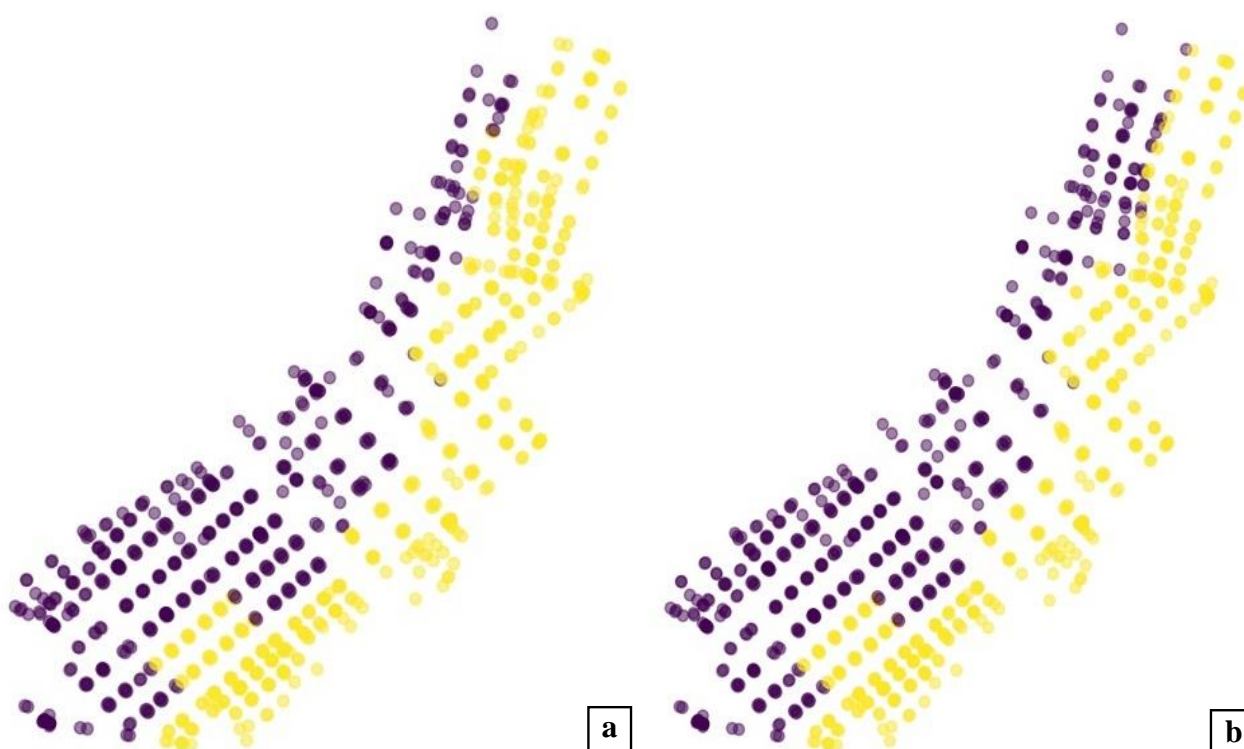
Figure 3. Partitioning of PMA “Kentro” into two clusters based on (a) nodal altitudes, and (b) simulated pressures.
