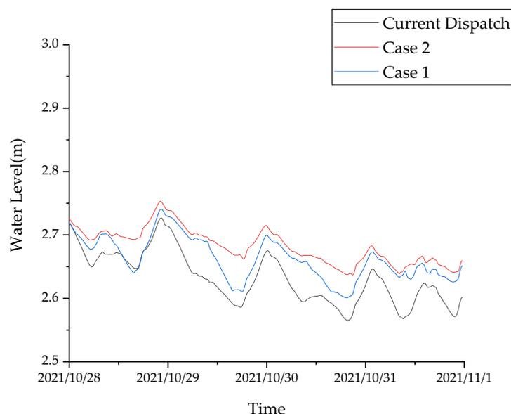
**Figure 10.** The process of water level in the internal riverway of the Qingsong Area under the current regulation and the two optimization schemes.
