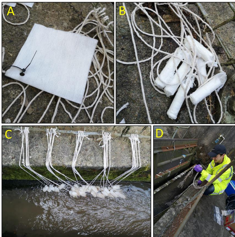
Fig. S5. Photographs showing (Panel A) the cotton (Moore) swab sampler, (Panel B) the tampon sampler, (C) deployment of the tampons in within the open wastewater channel, and (D) retrieval of a sampler after 24 h within the channel.
