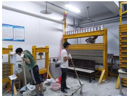
Figure 4. Laying process of the physical analog model.
