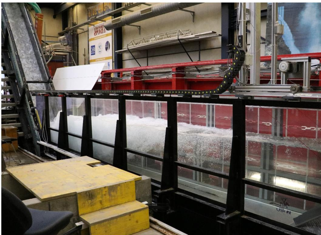
**Figure 2.** Photo of the spillway model with  $Q = 0.14 \text{ m}^3/\text{s}$ , the  $50^\circ$  smooth chute in the background and the plain stilling basin at the front. Flow direction from left to right.
