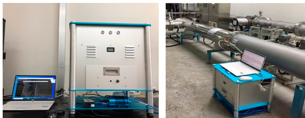
Figure 1. Portable •OH scavenging demand analyzer at UV/H 2 O 2 pilot plant.
