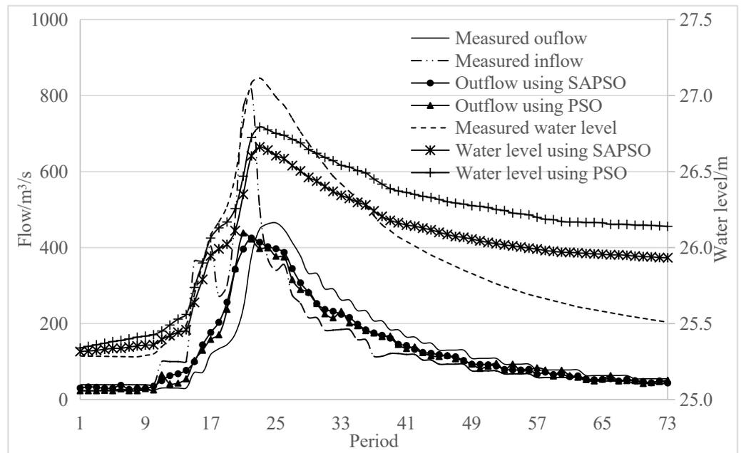
Figure 5. Operation hydrographs of Tianzhuang Reservoir for the 13 August 1974 flood.
