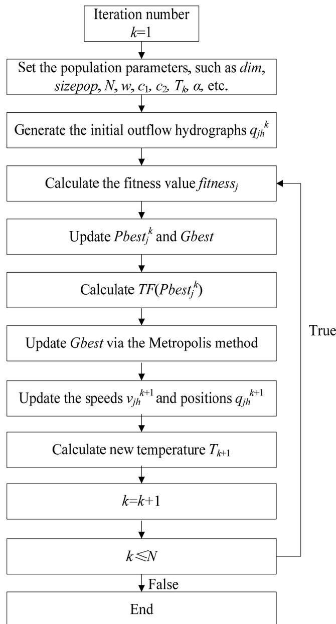
**Figure 1.** The flowchart of the procedure for determining optimal operation using the SAPSO algorithm.
