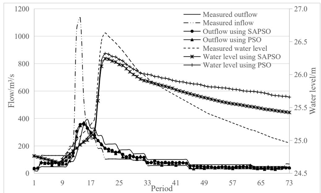
**Figure 3.** Operation hydrographs of Tianzhuang Reservoir for the 31 July 1964 flood.
