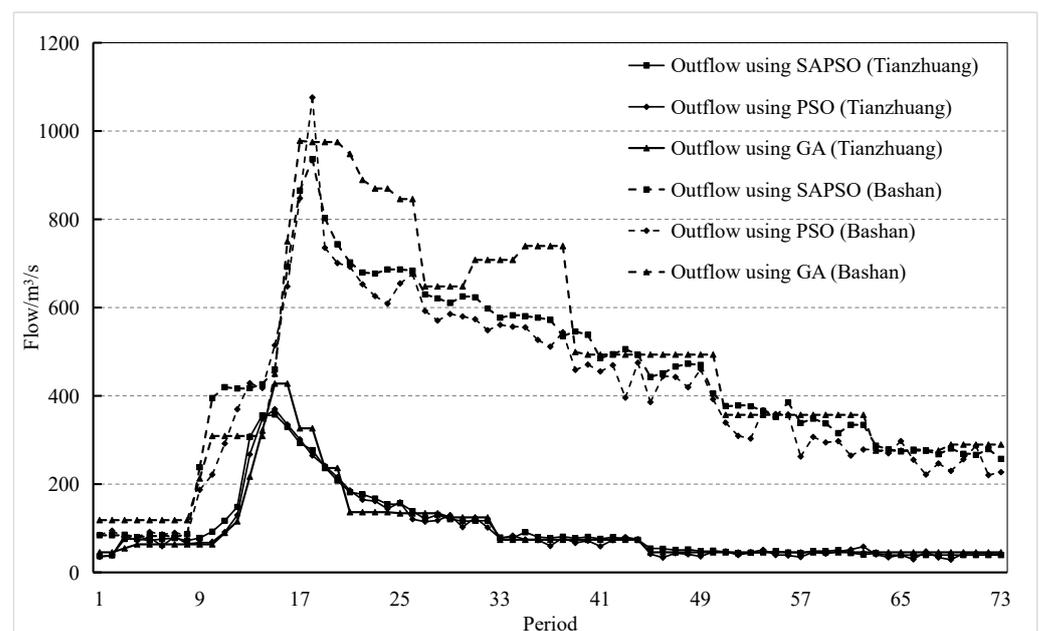
Figure 9. Outflow hydrographs for the 31 July 1964 flood using the SAPSO, PSO, and GA algorithms.
