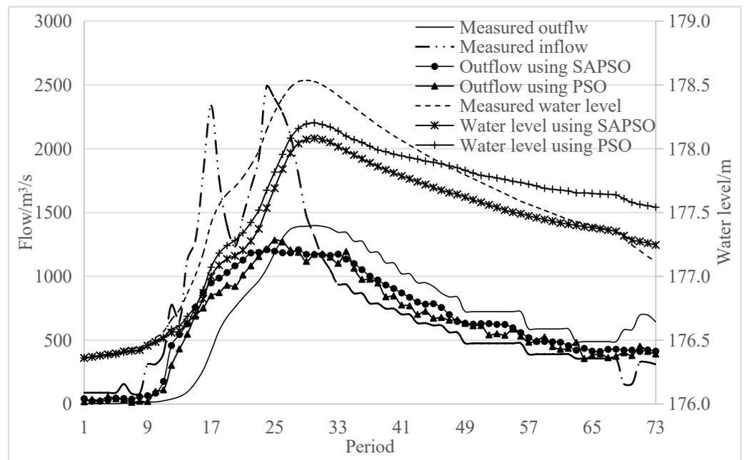
Figure 6. Operation hydrographs of Bashan Reservoir for the 13 August 1974 flood.
