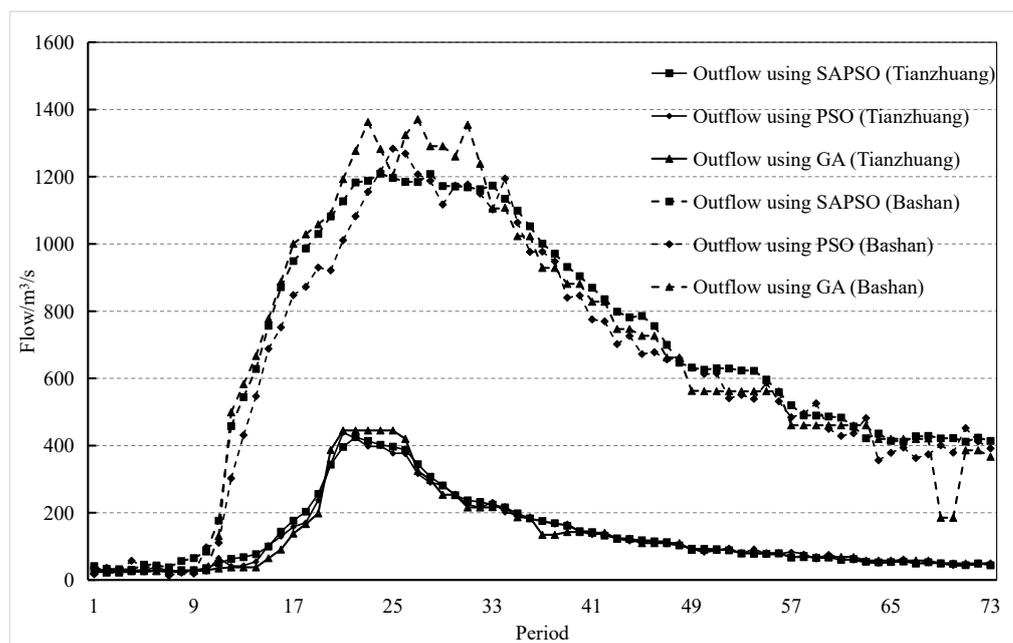
Figure 10. Outflow hydrographs for the 13 August 1974 flood using the SAPSO, PSO, and GA algorithms.
