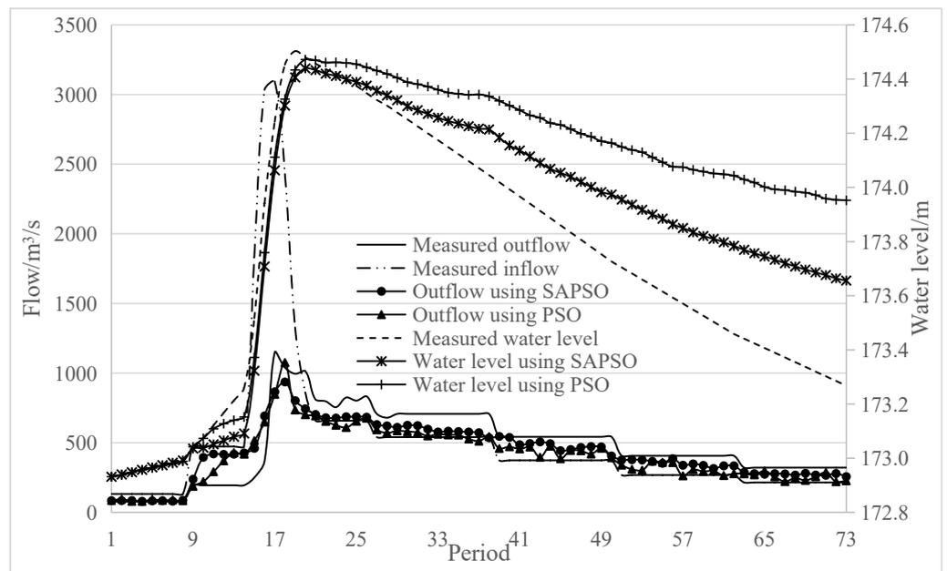
Figure 4. Operation hydrographs of Bashan Reservoir for the 31 July 1964 flood.
