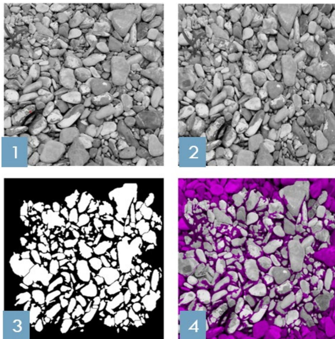
**Figure 4.** Graphical illustration of the key steps performed in the Digital Gravelometer software for the identification and measurement of different grain sizes: (1) Greyscaling; (2) projection transformation for camera adjustment; (3) grain selection; (4) greyscale image mask overlay on the selected grains in the previous step.
