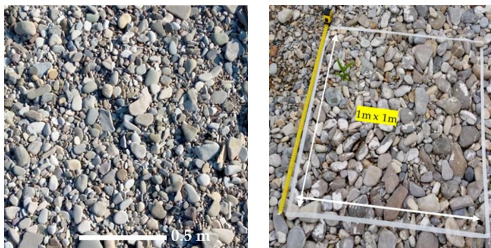
**Figure 2.** Digital photographs of the Baganza streambed taken for the grain size analysis using Digital Gravelometer.
