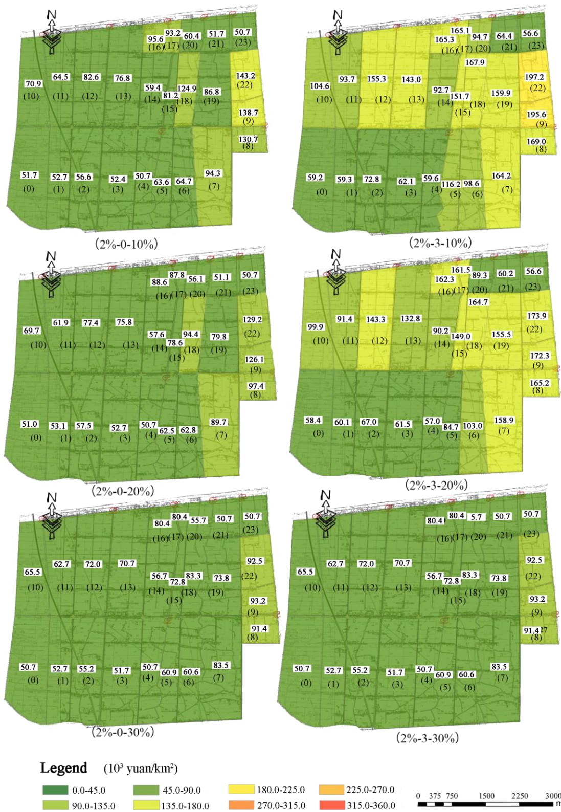
Figure 13. Distribution of averaged waterlogging loss with different initial storage depths and work scales under 2% frequency.
