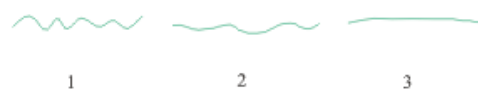
Figure 4. The morphology of contour for different Karst stages 1, 2, and 3 represent three Karst development stages from strong to weak degree.
