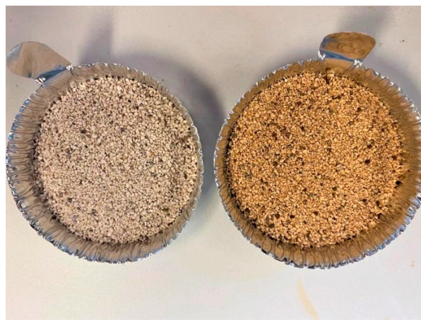
Figure 2. Physical appearance of natural and iron-coated zeolite.
