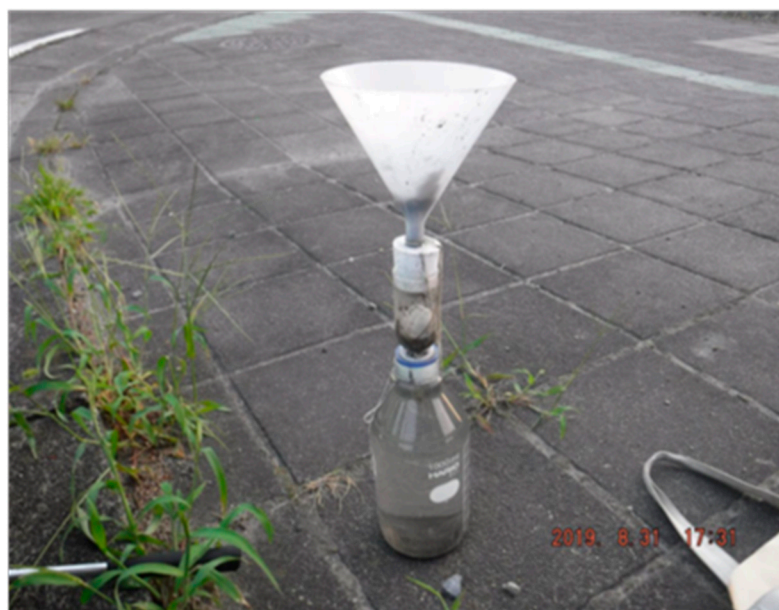
Figure 3. Water collection device.
