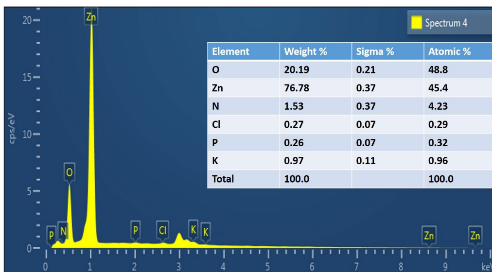
Figure 6. EDX spectrum and element ratio of green ZnO particles synthesized using Chrysanthemum spp. flower extract.
