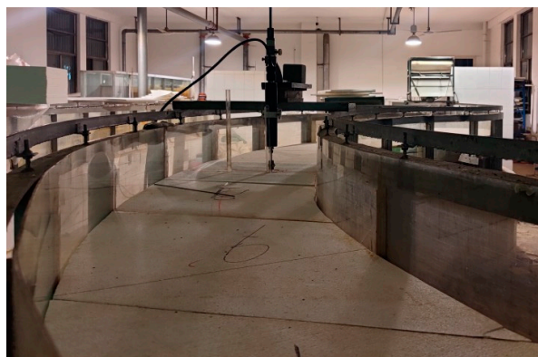
Figure 3. Measurement of flow velocities in front of the piers using an ADV.
