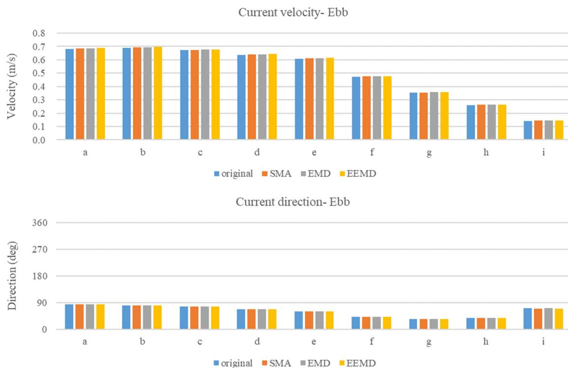
**Figure 16.** Flow velocity and direction distribution within the outer fairway to the breakwater (a-i) under ebb tide conditions.
