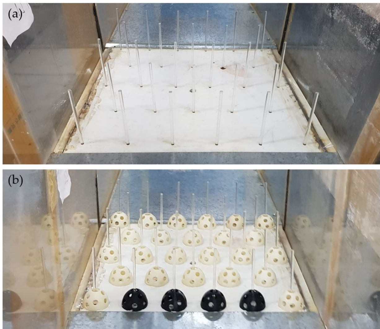
Figure 2. Arrangement of combining coastal trees with reef ball modules: (a) STDS, (b) RCDS.
