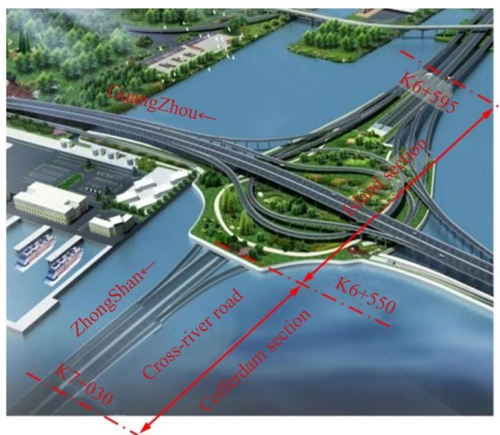
Figure 1. Plane position of the cofferdam.
