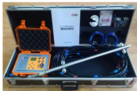
CX-3C inclinometer for foundation pit
