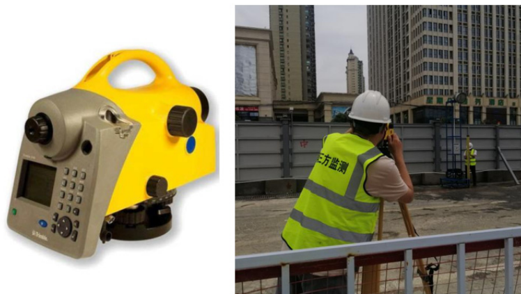
Trimble DINI03 electronic level Field picture of displacement monitoring
