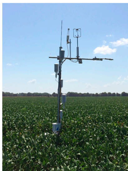
Figure 1. Eddy covariance unit with sensor cluster positioned 2 m above the canopy centrally located in a large farm-scale soybean field.
