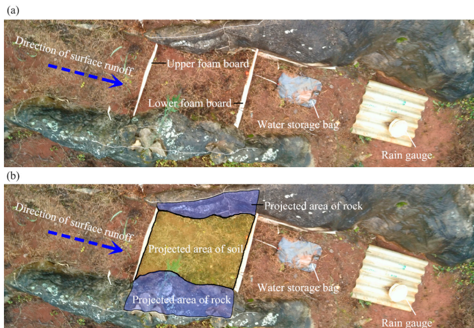
Figure 1. Design and implementation of the soil–rock combination runoff plot. (a) The placement of foam board, water storage bag, and rain gauge. (b) The projected area of the rock and the soil patch of the soil–rock combination runoff plot.
