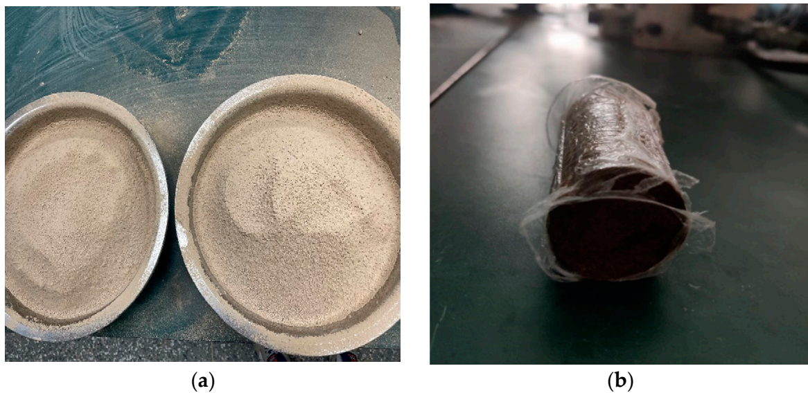
Figure 2. Procedure for preparing test soil samples (a) Crushed and sieved soil; (b) Partially fabricated specimen.
