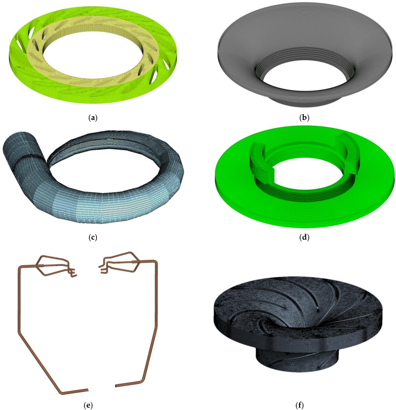
Figure 3. Mesh division of each part: (a) Mesh of the double row cascade; (b) Mesh of the lower ring gap; (c) Mesh of the spiral casing; (d) Mesh of the upper crown gap; (e) Mesh of the flat pressure tube; (f) Mesh of the runner.
