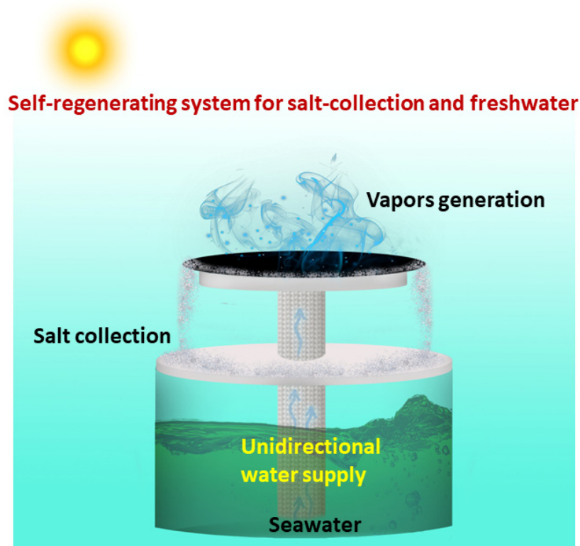
Figure 1. Illustration of a solar evaporation system for simultaneous salt and freshwater production.
