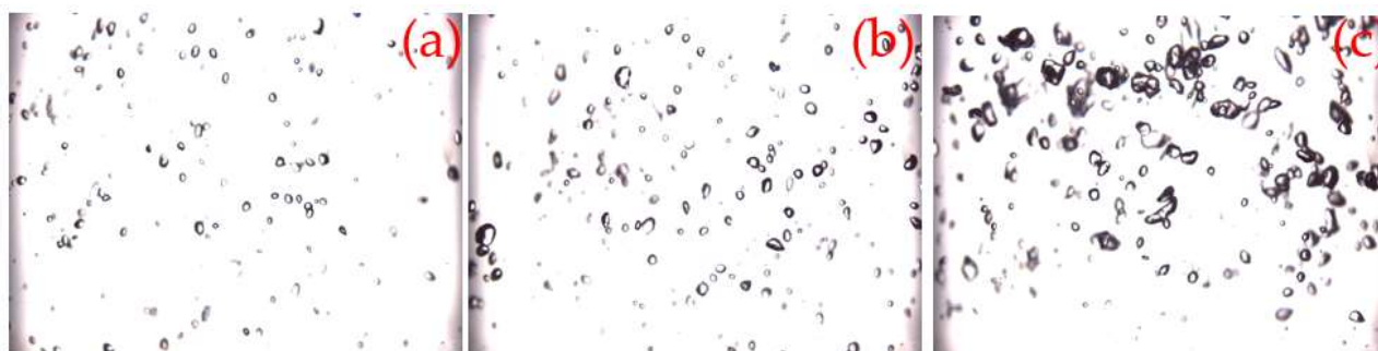
Figure 6. Distribution of bubbles with different air contents: (a) 0.05 air content; (b) 0.1 air content; (c) 0.15 air content.
