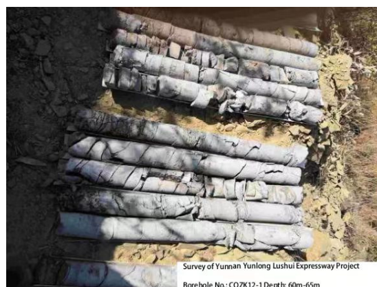
Figure 3. Deep stratigraphy of Yunlong side bank slope.
