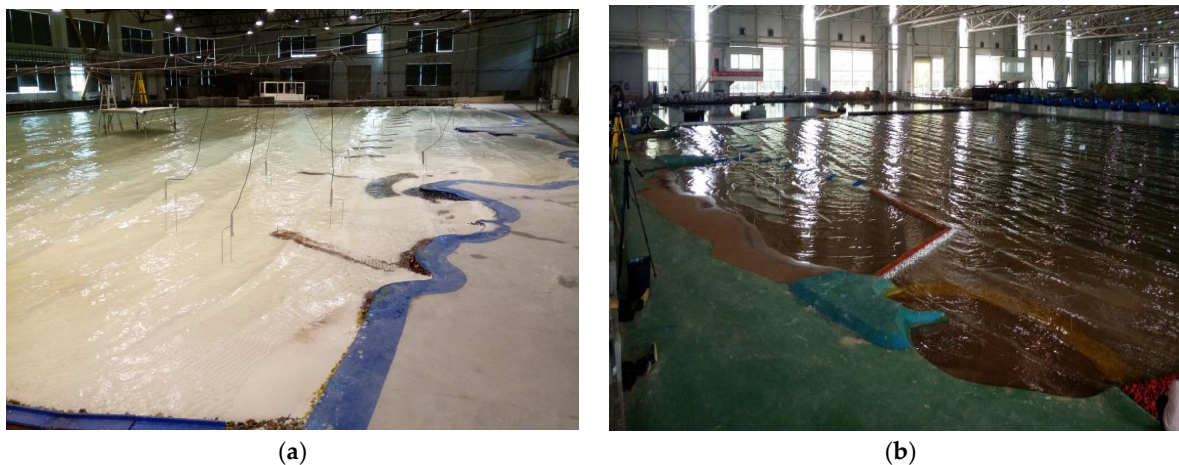
Figure 2. Part of the results of research on beach protection measures in the laboratory: (a) combination test of spur dike and submerged dike; (b) combination test of sand barrier and submerged embankment.
