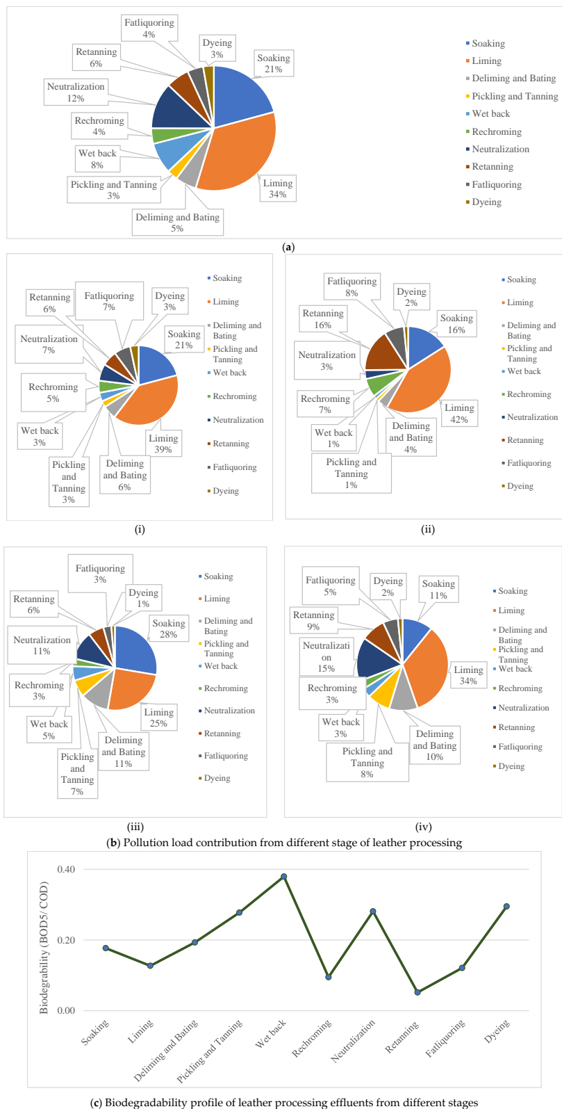
Figure 6. Volume and characteristics of effluent generated by different stages of leather processing. (a) Effluent generation from leather processing stages. (b) Pollution load contribution from different stages of leather processing: (i) BOD, (ii) COD, (iii) TDS and (iv) TSS. (c) Biodegradability profile of leather processing effluents from different stages.
