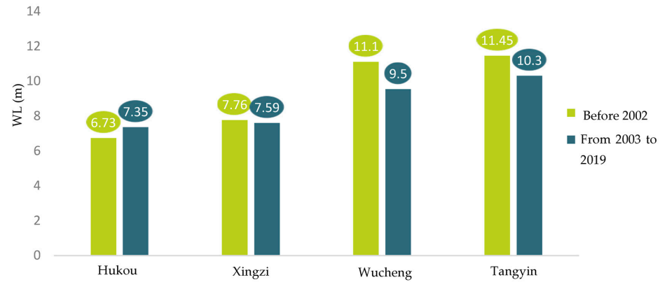
Figure 8. Change of the water level with a 98% guarantee rate of duration at the main hydrometric stations in the lake area in different periods.
