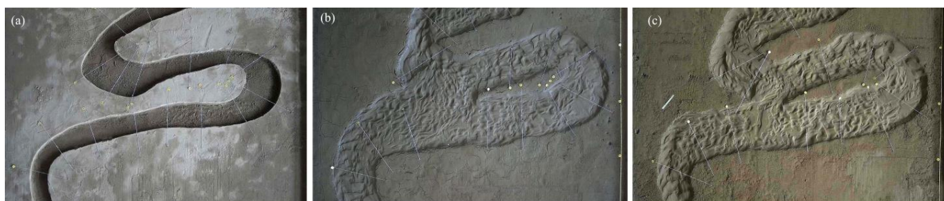
Figure 9. Comparison between (a) the initial terrain and the final terrain after cutoff with (b) the topography of the relative equilibrium in RUN2 and (c) the topography of the relative equilibrium in RUN3. The white line represents the measured cross section. The yellow line on the right marks the length.
