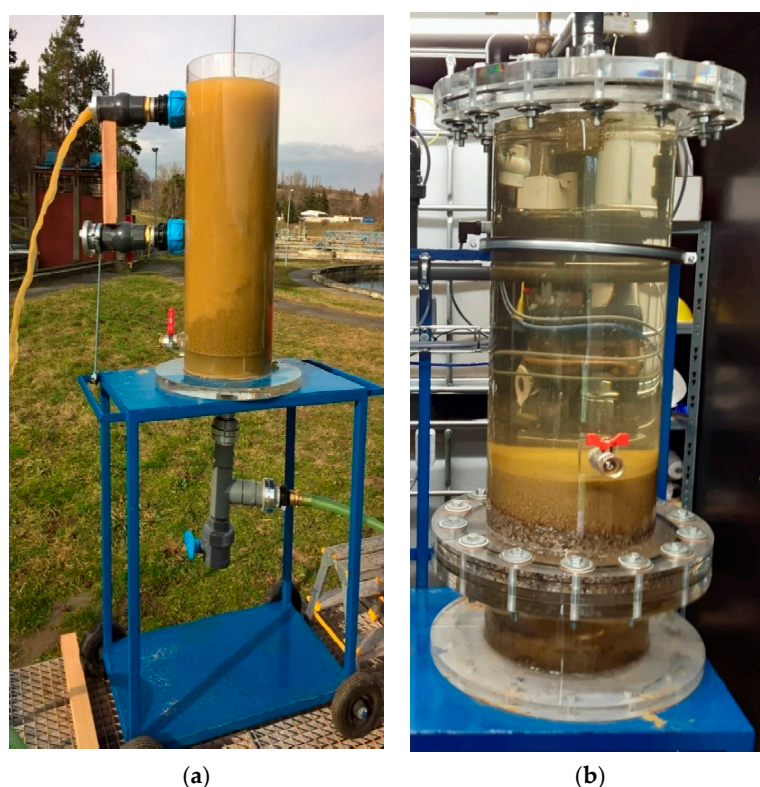
Figure 8. (a) Photo of a column for hydrodynamic treatment of Bentonite Branany EXTRA; (b) photo of developed pilot plant sorption unit for microplastics capture tested in the municipal WWTP in the Czech Republic.
