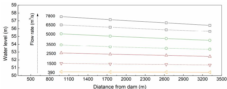
**Figure 8.** Water surface curve distribution downstream of the dam at different flow rates.
