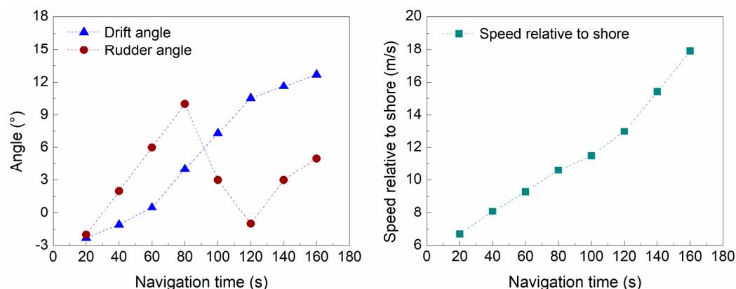
**Figure 16.** Change process of ship navigation parameters with navigation time at a typical flow rate ( $Q = 6500 \text{ m}^3/\text{s}$ ).
