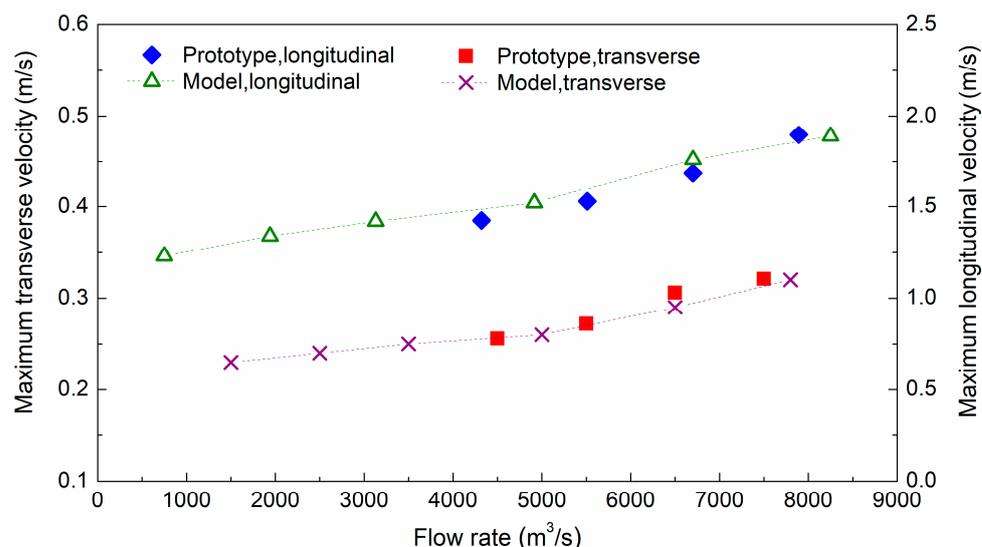
Figure 15. Comparison of extreme values of the surface flow velocity at the entrance area of the approach channel between the prototype and the model.
