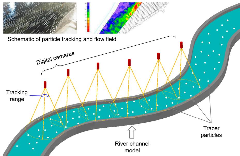
**Figure 6.** Schematic of the flow-field real-time measurement system (VDMS).
