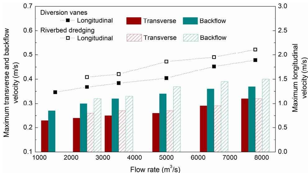
Figure 13. Comparison of navigable flow conditions between optimal riverbed-dredging and optimal diversion vanes schemes.
