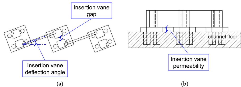
**Figure 3.** Schematic of the diversion vanes structural parameters. (a) Plan view; (b) side view.
