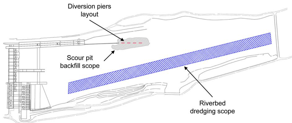
Figure 12. Schematic of optimal arrangement of riverbed-dredging scheme.
