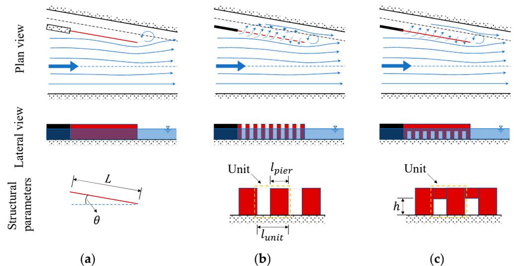
**Figure 1.** Schematic of three types of existing diversion structures. (a) Navigation wall, (b) diversion piers, and (c) partition dykes.
