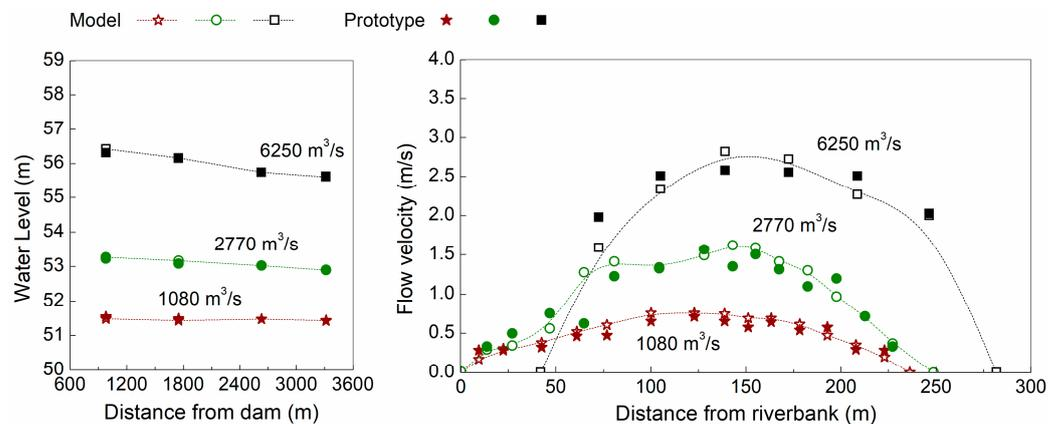
**Figure 7.** Comparison of water level and cross-section flow velocity between the prototype and the model.
