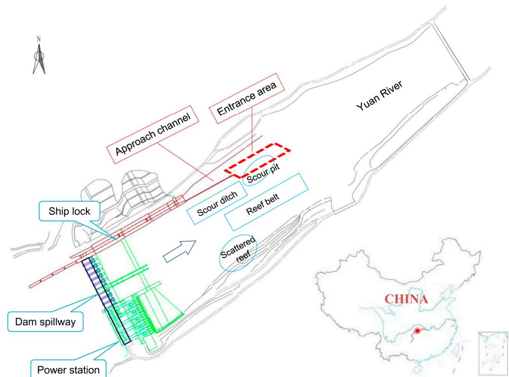
**Figure 4.** Location and layout of the Wuqiangxi hydro-junction.
