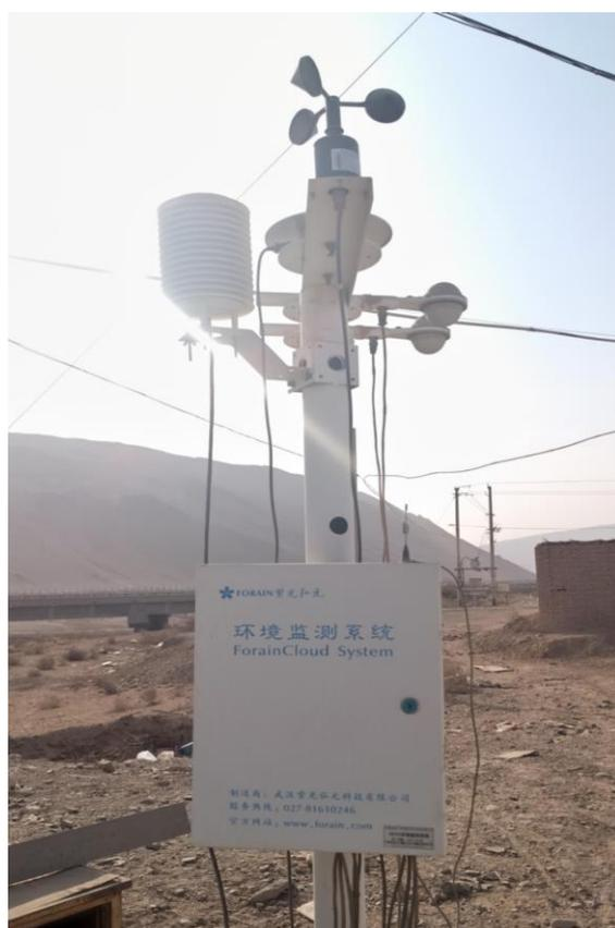
**Figure 6.** Automatic weather station used in the test. Note: The meaning of Chinese in the figure includes brand of weather station, equipment name, corporate name, contact telephone and official website address.
