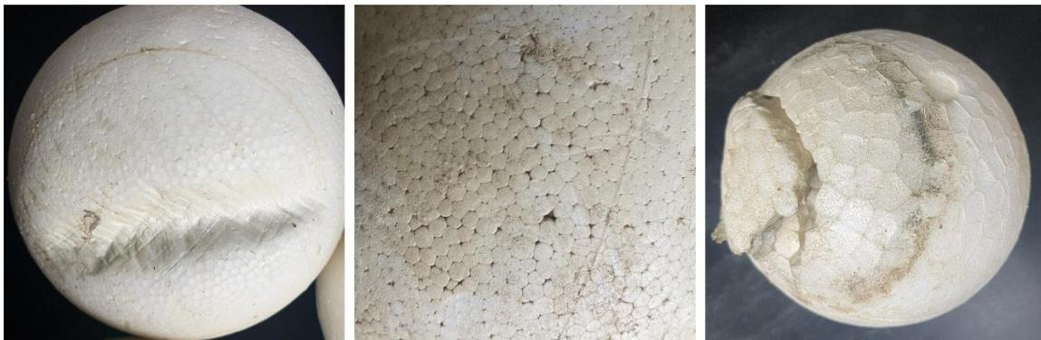
**Figure 12.** Common failure modes of EPS balls.
