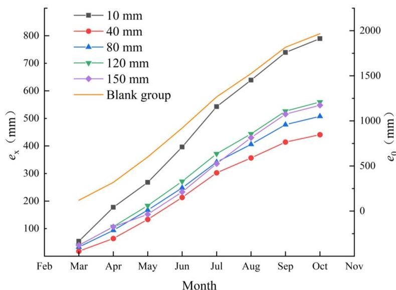
**Figure 7.** Cumulative evaporation capacities of all evaporators for different diameter balls.
