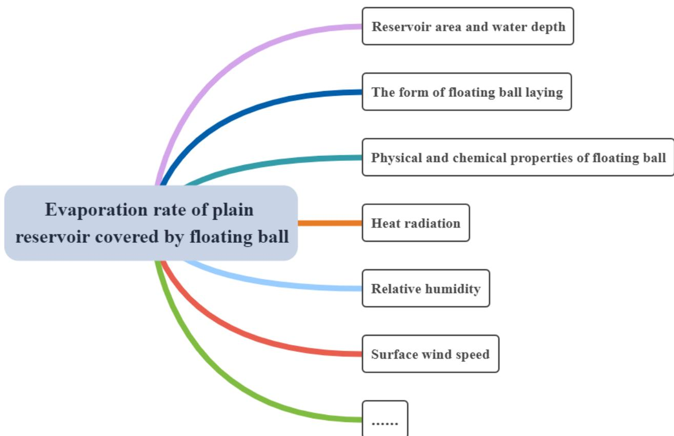
**Figure 3.** Main influencing factors of evaporation rate of plain reservoir covered by floating balls. Note: “.....” indicates other factors affecting evaporation rate in small-sized water bodies, but their importance is weaker in reservoirs.
