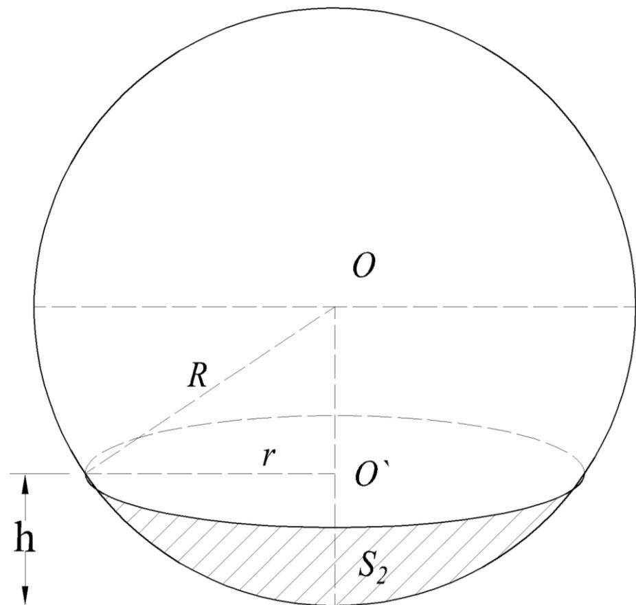
**Figure 11.** Schematic diagram of spherical crown calculation.
