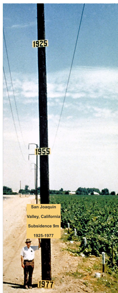
Figure 2. The maximum vertical deformations in the San Joaquin Valley, California. The signs on the column were placed at the approximate former altitudes of the earth's surface between 1925 and 1977 [56].
