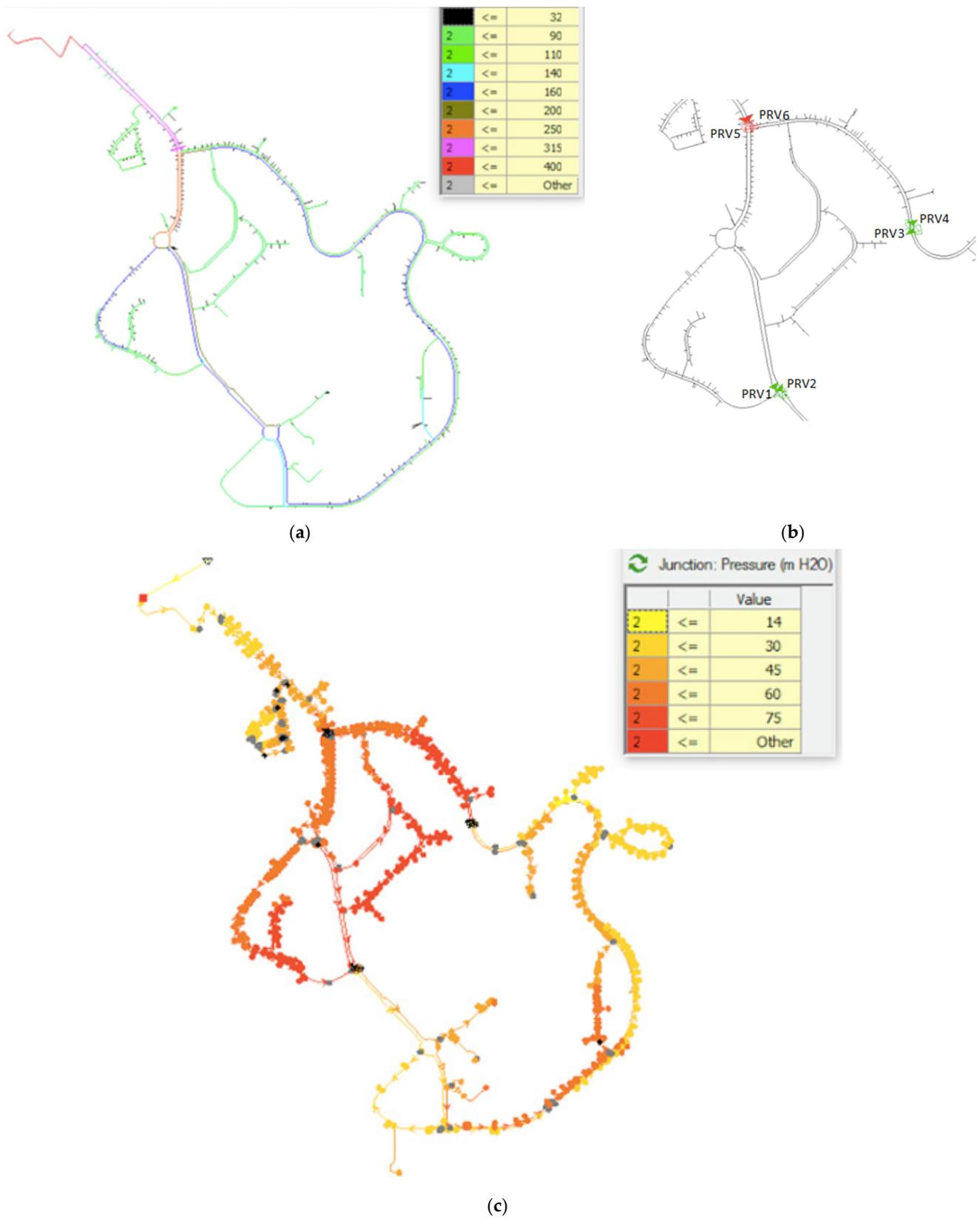
**Figure 10.** Diameter range of the water network under study (a); Localization of PRVs (b); pressure distribution in the WDN of Beloura (c).
