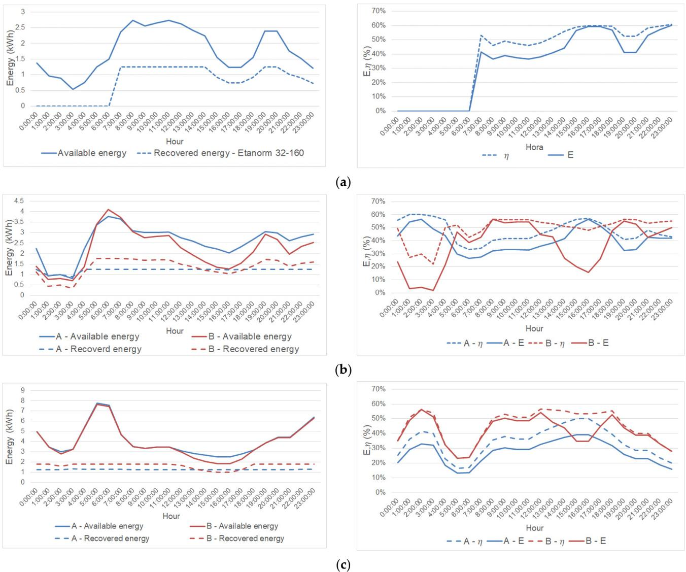
**Figure 14.** Available and recovered energy for different demand patterns type (left) and effectiveness (E) and capability ( $\eta$ ) (right): (a) normal; (b) high; (c) very high consumption scenarios.
