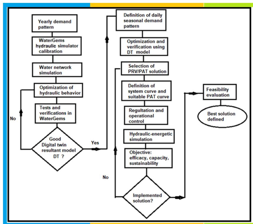
Figure 3. Flow-chart of the proposed integrated efficiency management methodology.
