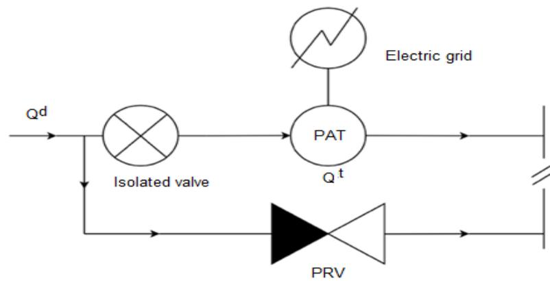
Figure 12. PAT installation scheme.
