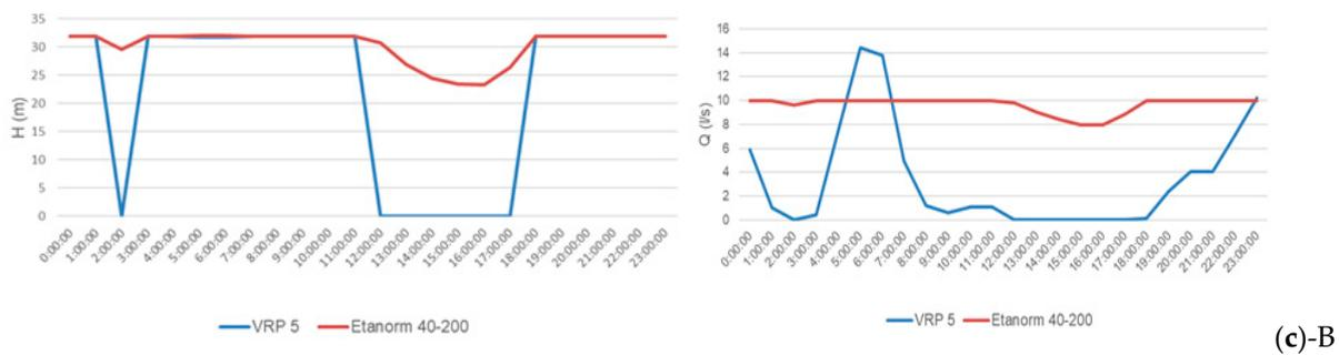
**Figure 13.** Hourly head and flow for: (a) normal; (b) high (with alternatives A-PAT1 and B-PAT1+2) and (c) very high (with alternatives A-PAT1 and B-PAT2) demand periods.
