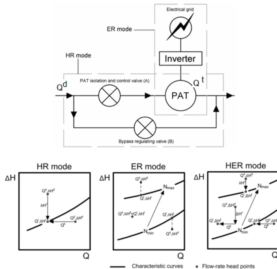
**Figure 1.** Hydraulic regulation (HR), Electrical regulation (ER) and (Hydraulic-Electrical regulation (HER) modes).
