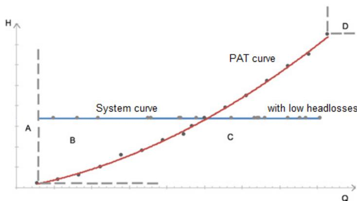
Figure 4. Possible operating zones when a PAT is installed within the system.
