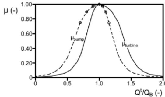
Figure 2. Standard reliability curves, pump and turbine modes [24].
