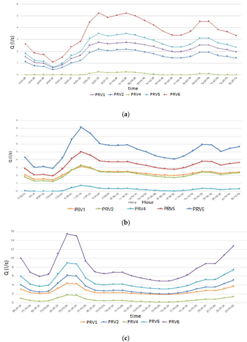
**Figure 11.** Flow rates within PRVs for different demand consumptions: (a) normal consumption; (b) high; (c) very high.
