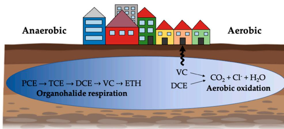
**Figure 1.** CEs degradation pathways. In the anaerobic portion, there has been incomplete reductive dechlorination with the accumulation of DCE and VC (dashed arrows). Following the aerobic portion permits complete mineralization of the pollutants.
