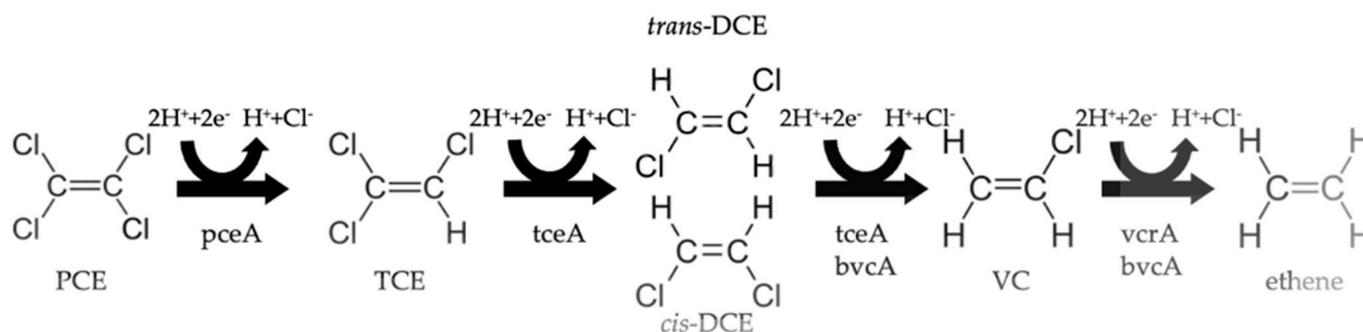
**Figure 2.** Anaerobic respiration pathway: organo-halide dechlorination of PCE to ethene and respective enzymes involved in the process: PCE reductase pceA, TCE reductase tceA, DCE/VC reductases bvcA, and vcrA. Modified from [35].
