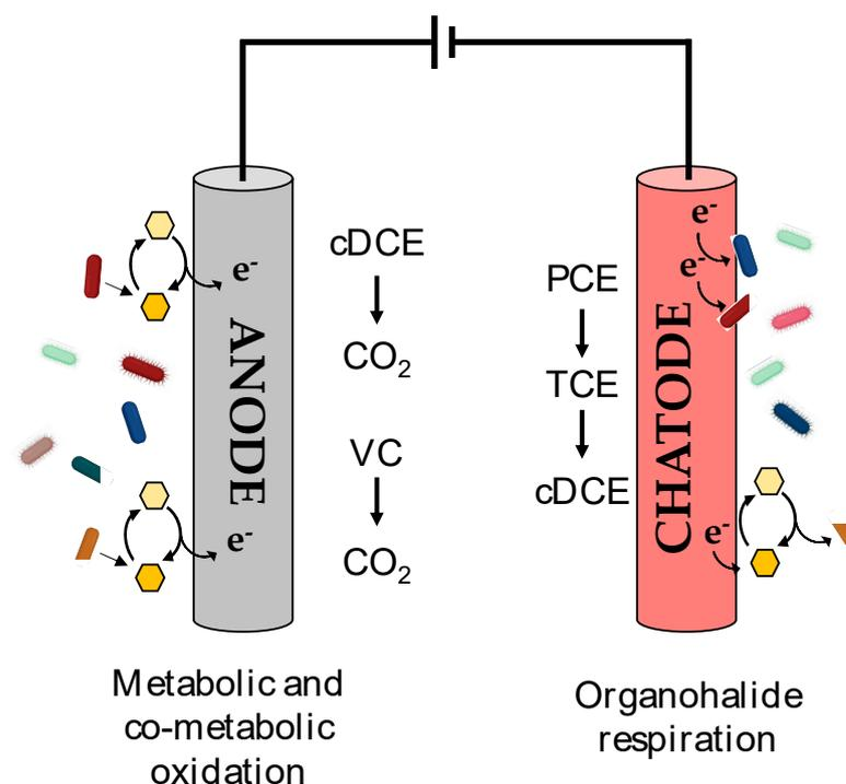
**Figure 6.** Illustration of a bioelectrochemical cell with aerobic and anaerobic biotransformation of chloroethene mechanisms.
