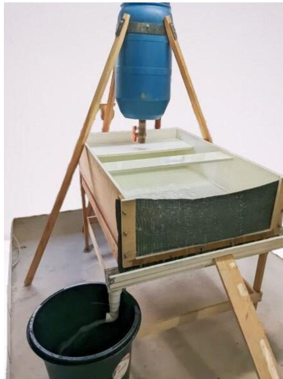
Figure 1. Photo of the apparatus used in this study with the geotextile assembled.
